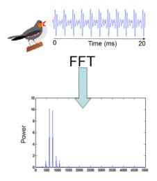
Each of of the peaks in the Power Spectrum above, corresponds to a sine wave, e.g.,:
